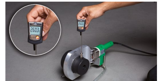
Temperature control aquatherm welding device (1400 W)
