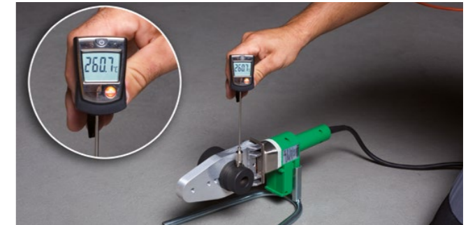
Measurement of temperature at the aquatherm manual welding device (800 W).
