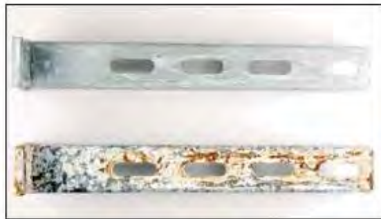
Cantilever Bracket 41/41 after 1,440 h salt spray test; Above: zinc-lamella coated Below: zinc-galvanised
