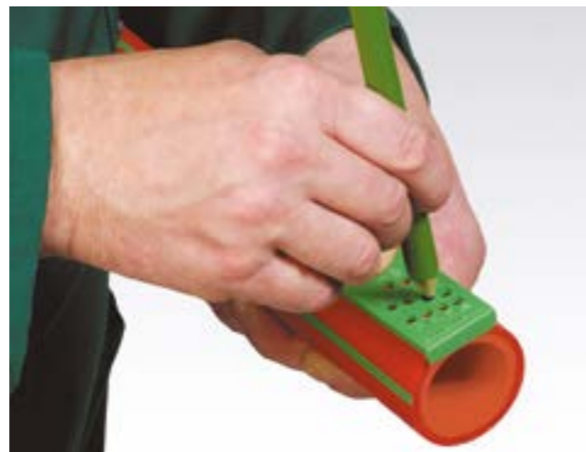
Marking of the welding depth
