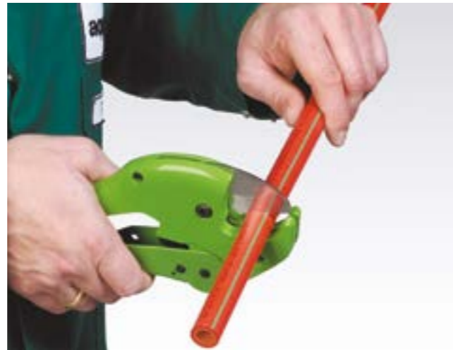
Cutting of the pipe
