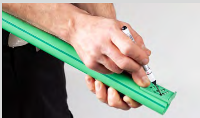
Marking of the welding depth
