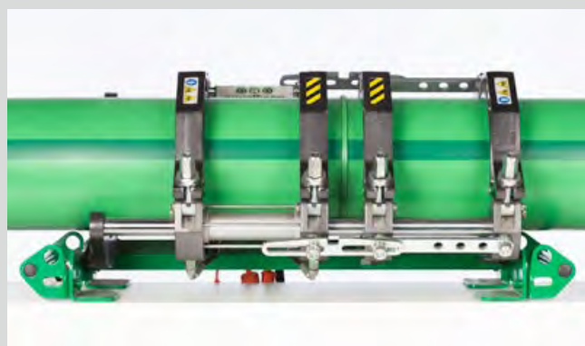
Join the pipes, cool down under pressure
