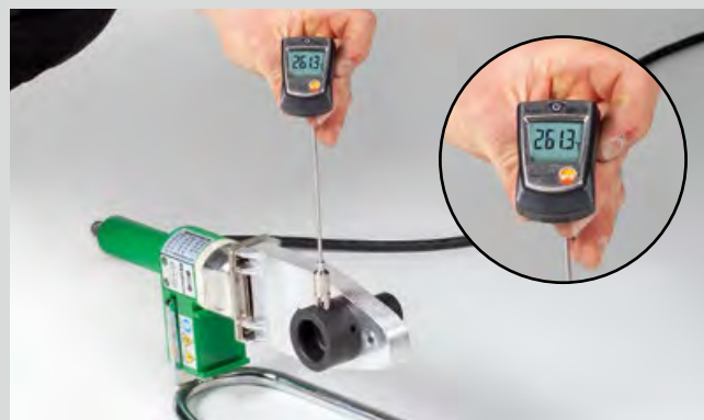
Measurement of temperature at the aquatherm manual welding device (800W )
