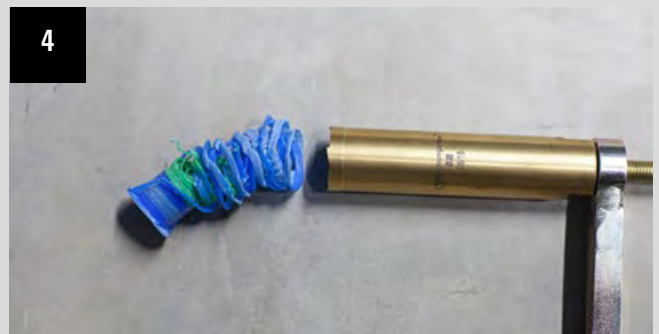
4. Removal of the drilling residues out of the drilling tool
