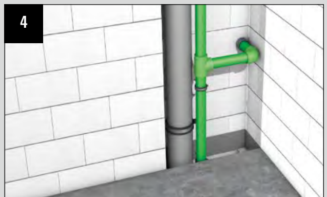
Installation of a spring leg
