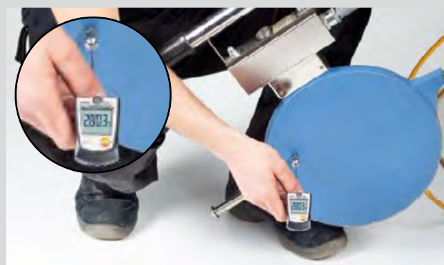
Measurement of temperature at the aquatherm butt-welding machine
