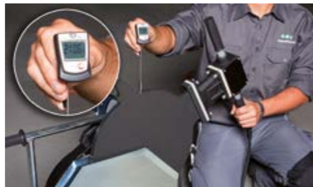
Temperature measurement on aquatherm butt fusion machine
