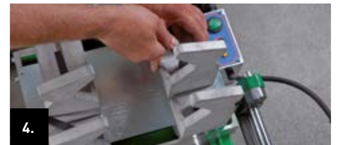
4. Slide the rear pair of clamping jaws for pipe fastening onto the front pair of clamping jaws and secure by tightening the fastening screws.
