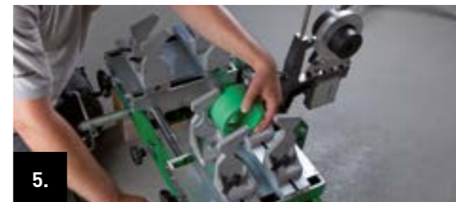
5. Hold the welding socket between the moulded part clamping jaws and press against the stops on the end face.
