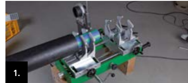
1. Set up and align the welding machine. Take space requirements into account! (Please note that the machine must be removed from underneath the pipe after welding work has been completed )
