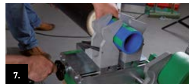
7. Push the pipe end between the clamping jaws and centre it by turning the crank handle, but do not tighten it.
