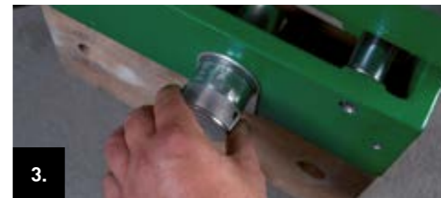
3. The welding depth of the pipe dimension to be processed is set using the rotary knob (on the left front of the machine frame).
