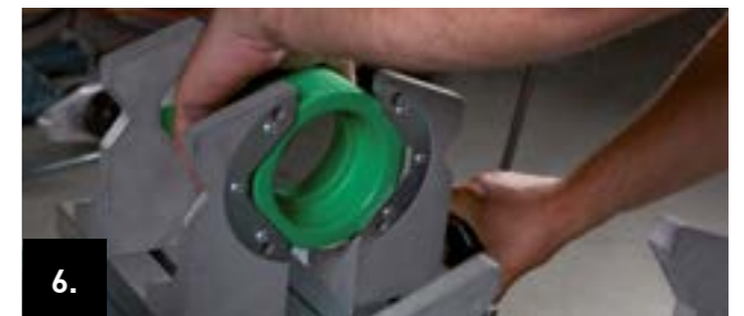
6. Fix the sleeve against the stop and tighten the clamping jaws firmly with the crank handle .
