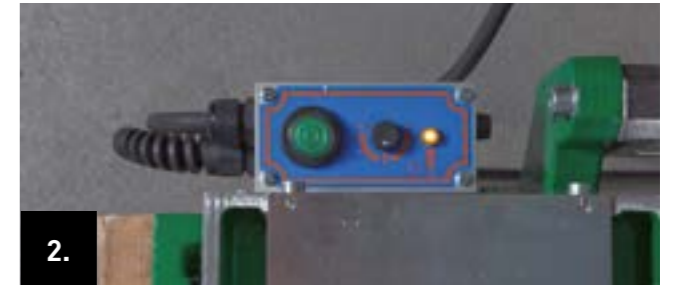
2. Connect the power supply and check whether the yellow operating indicator lights up.
